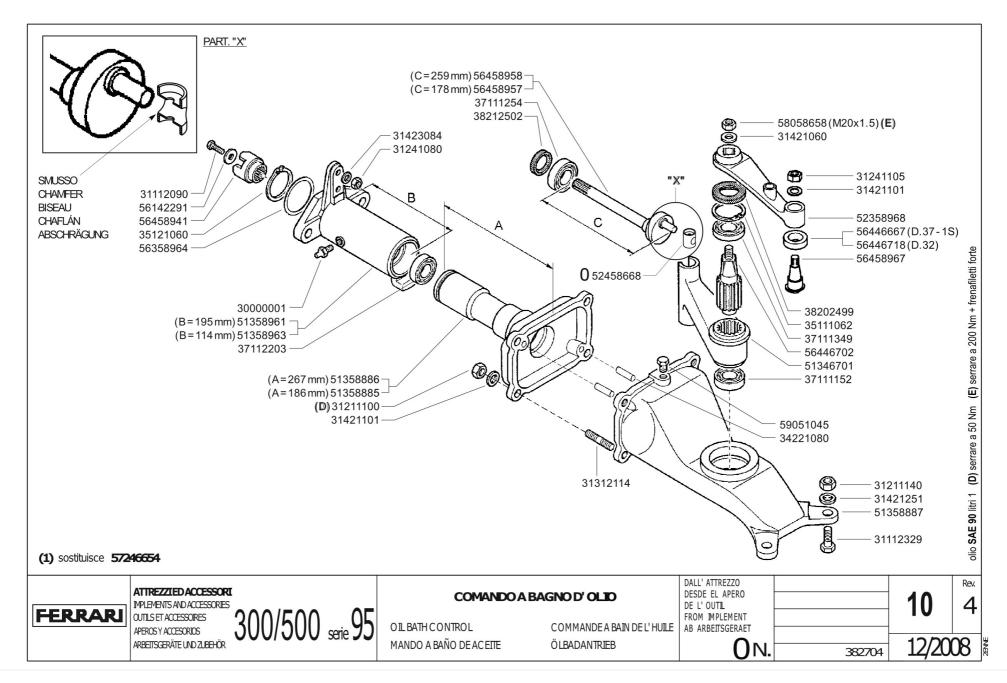
FERRARI Motor mowers, FERRARI 2-wheel tractors - TRANSMISSION IN OIL BATH
